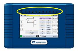
In case of auxiliary power supply failure, the status of the leds is recorded and reproduced when power supply is restored.
