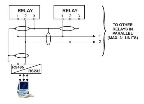
For longer distance and for connection of up to 250 Relays, optical interconnection is recommend. (please ask Microelettrica for accessories)
