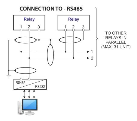
For longer distance and for connection of up to 250 Relays, optical interconnection is recommended. (Please ask Microelettrica for accessories)
