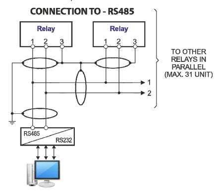
For longer distance and for connection of up to 250 Relays, optical interconnection is recommend. (Please ask Microelettrica for accessories)
