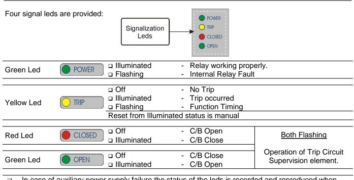
In case of auxiliary power supply failure the status of the leds is recorded and reproduced when power supply is restored.
