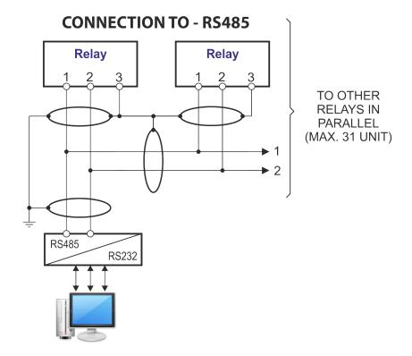
For longer distance and for connection of up to 250 Relays, optical interconnection is recommended. (Please ask Microelettrica for accessories)
