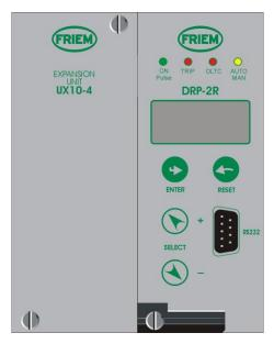
The regulator can be managed locally, either by the RS232 communication port or by the 4 key buttons and the LCD display. The regulator is also managed via the communication bus RS485 at the rear terminal blocks. The 2 line x 8 characters LCD display shows the available information. Key buttons operate according to flow-chart here below.
