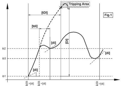
If during [tDI] the rate of rise "di/dt" goes below the set level [di] for a time longer than [tdi], a new value of the current  $i_{b2}$  is recorded and, when [tDI] expires. If the difference " $\Delta I = i - i_{b2}$ " measured is greater than [DI], the protection function trips.
