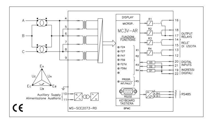
With this connection, the secondary rated voltage of the PT (see wiring diagram) must be set at the rated phase-to-phase voltage multiplied by 1.73.
