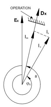
The overcurrent element operates in a real directional mode measuring the component "ldx" of the input current in the reference direction "a" (x = A, B, C).
