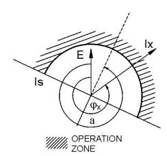
The Overcurrent element only supervises the direction of the current:
