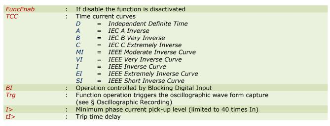
Trip when : The current trip level is exceeded for time "tI>".
