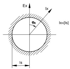
The overcurrent element operates independently from the current direction.
