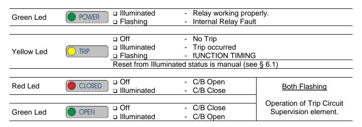
□ In case of auxiliary power supply failure the status of the leds is recorded and reproduced when power supply is restored.
