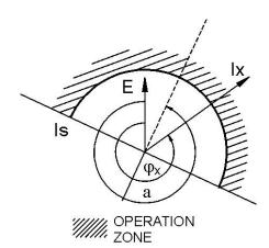
The Overcurrent element only supervises the direction of the current:
