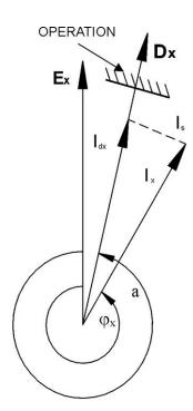
The overcurrent element operates in a real directional mode measuring the component "Idx" of the input current in the reference direction "a" (x = A, B, C).
