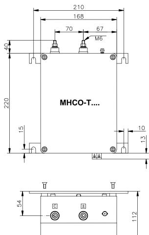
B) Receiver unit – Surface mounting on profile DIN-EN50022
